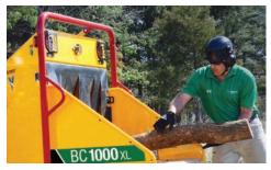
**OPERATOR SAFETY.** Combined with the patented bottom feed stop bar is the four-position upper feed control bar with dual stop positions and forward/reverse feed positions. Mounted over the feed table, it enables the operator to stop the feed rollers and select forward or reverse operations. Dual reset/hold-to-run buttons allow the operator to readily reset the bottom feed stop bar.
