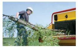
**SMARTFEED.** The patented SmartFeed system helps increase operator productivity while reducing strain on vital engine parts. The feedsensing control system monitors engine rpm and automatically stops and reverses the feed roller when feeding larger, hardwood material.
