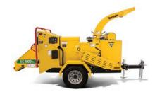
**CLUTCHLESS PTO.** The throttle integrated with the belt drive engagement process helps ensure that the PTO can only be engaged while the engine is at low idle/low rpm. Automatically, the engine throttles up to full rpm after the belt drive is fully engaged. This system helps to reduce premature wear to the belt drive system by preventing high idle engagement of the cutter drum.
