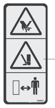
Moving blades/blade arms cut/crush Hazard
