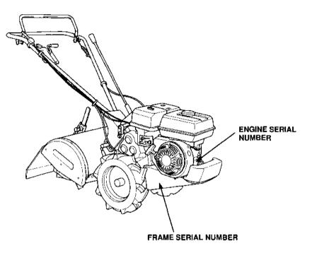
Record the engine and frame serial numbers in the spaces below. You will need this serial number when ordering parts, and when making technical or warranty inquires (see page 64).
