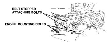
During adjustment, line up the groove of the engine-side pully and thet of the transmission-side pulley. If they are not aligned, the belt may come off or will wear prematurely.
