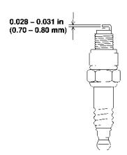
If reinstalling a used spark plug, tighten 1/8 - 1/4 turn after the spark plug seats.
