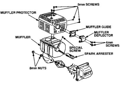
3. Use a brush to remove carbon deposits from the spark arrester screen. Be careful to avoid damaging the screen.
