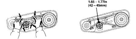
2. To adjust, loosen the four engine mounting bolts and the belt stopper attaching two bolts (front side) and move the engine forward or backward to get proper tension on the belt.
