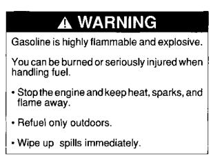
Refuel in a well-ventilated area before starting the engine. If the engine has been running, allow it to cool. Refuel carefully to avoid spilling fuel. Do not fill the fuel tank above the fuel level mark. After refueling, tighten the fuel tank cap securely.
