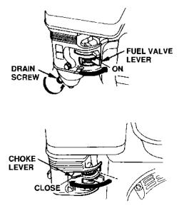
2. Move the choke lever to the CLOSED position to start a cold engine.
