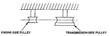
3. Loosen the belt stopper attaching bolts. Adjust the clearance between the belt stopper and the belt as illustrated with the clutch lever squeezed.
