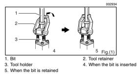
Pivot the tool retainer back and slightly downward. Insert the bit into the tool holder as far as it will go. To securely retain the bit, return the tool retainer to its original position.
