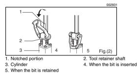
Pivot the tool retainer front and slightly downward. With the notched portion of the bit facing the tool retainer shaft, insert the bit into the tool holder as far as it will go. Then pivot the tool retainer further downward toward the cylinder to securely retain the bit.
